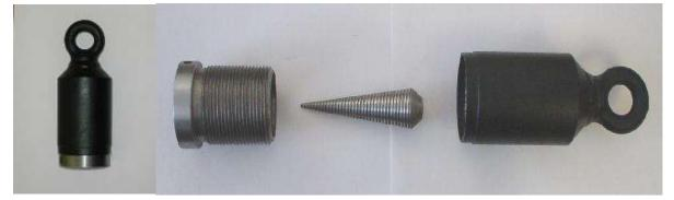
CLP's screw-on cable hauling eye is designed to offer maximum gripping strength on cable conductors of all types and conductor sizes 25-55mm diameter and suits all cable with an inner core. A short extension sleeve covers and protects the face of the cable insulation during hauling. The CER hauling eye provides an excellent grip to the cable by attaching directly to the cable conductor and can be fitted in the filed & best of all, no special tools required.
